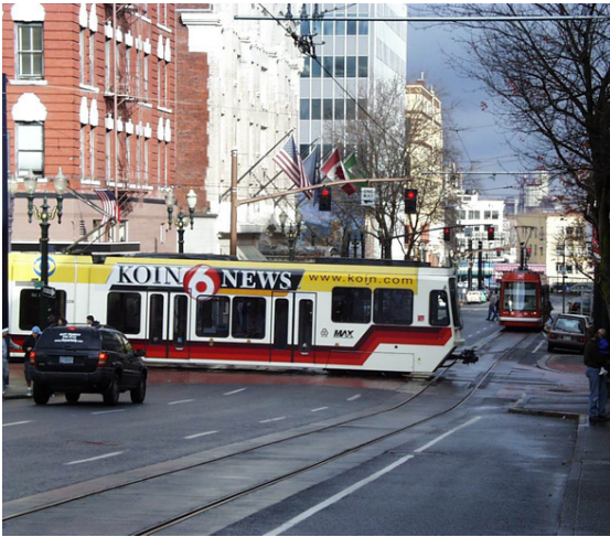
Figure X. “Light” rail Portland Max vehicle operating like streetcar in the foreground with a true light rail streetcar in the background.
